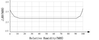
Figure 2: 25 °C relative humidity of maximum error AM2301
