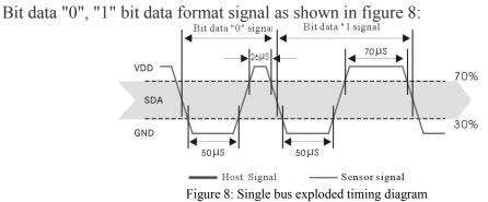
AM2301 SDA output data bus 40 data, continues to output low 50 microseconds and changed the input state, due to the pull-up resistor subsequently goes high. Meanwhile AM2301 environmental temperature and humidity inside the test-retest data, and record data, test recording ends, the microcontroller automatically goes to sleep. Only after receiving the start signal microcontroller host, only to re-awaken the sensor into working condition.
