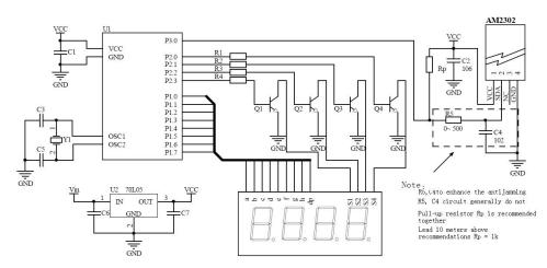
Figure 4: AM2301 single bus typical circuit
