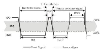
Figure 7: Single bus exploded timing diagram
