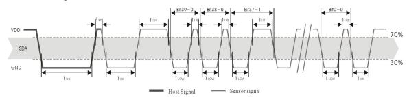
Figure 6: AM2301 single bus communication timing
